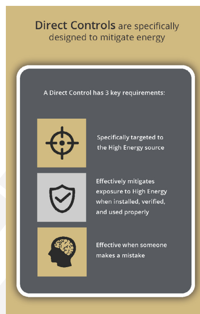
Figure 8: CSRA, direct controls requirements
