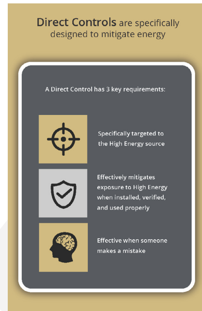
Figure 7: CSRA, direct controls requirements
