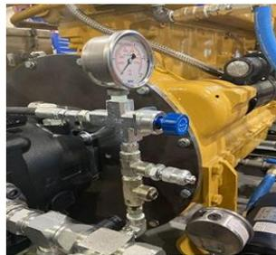
Recommended pipe configuration for pressure gauge isolation.
