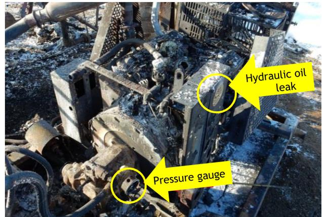
Burned engine: location of pressure gauge and oil leak
