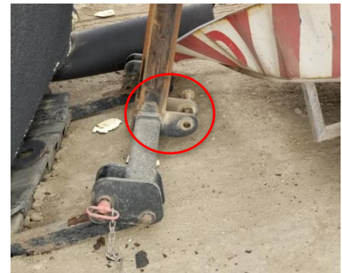
Close-up of the failed bracket with the Main mast pin out of position
