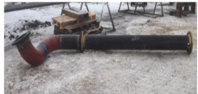
Example of pipe dropped off stands
