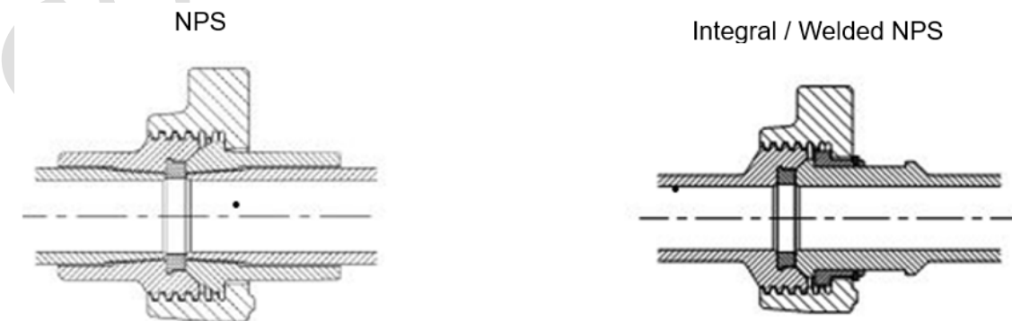
Figure 15. Hammer Unions High Pressure Containing Components (HPCC) Construction Types
