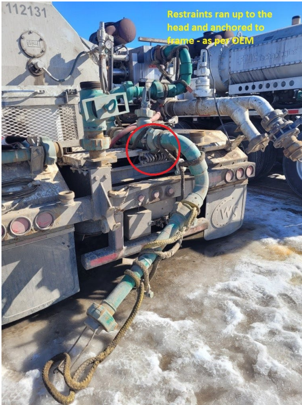
Figure 33. Fracture Pump Bridle with Restraints
