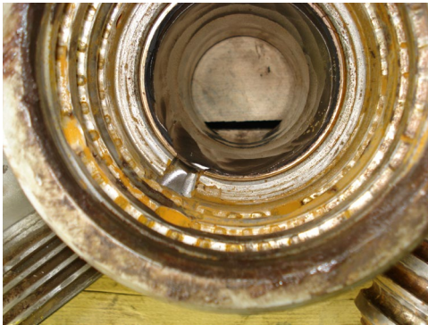
Figure 29. Washed Out Swivel
