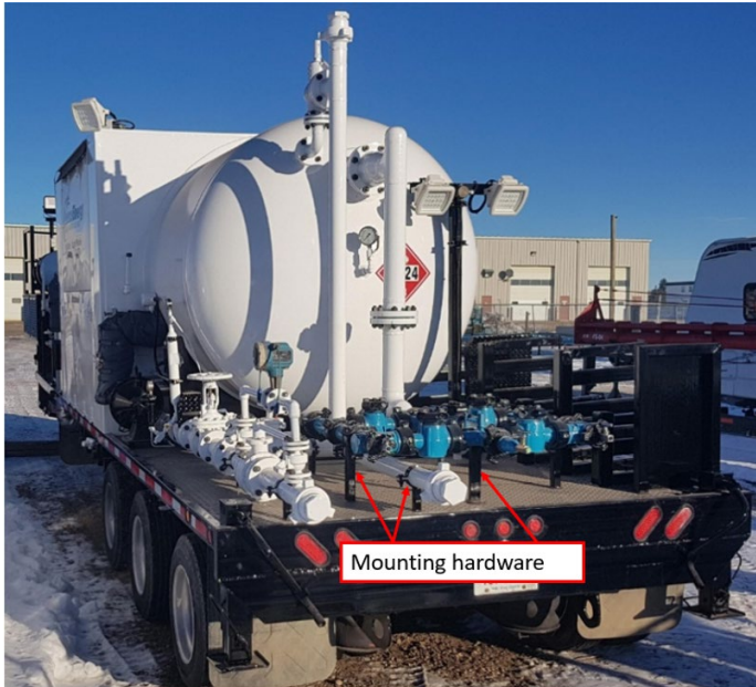
Figure 30. Example of Mounted Pipework
