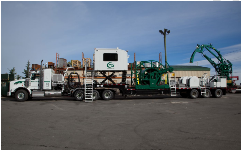
Figure 53. Coiled Tubing Unit
