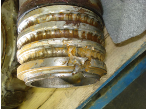
Figure 29. Washed Out Swivel
