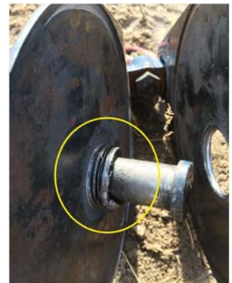
Damage to snatch block, evidence of side loading
