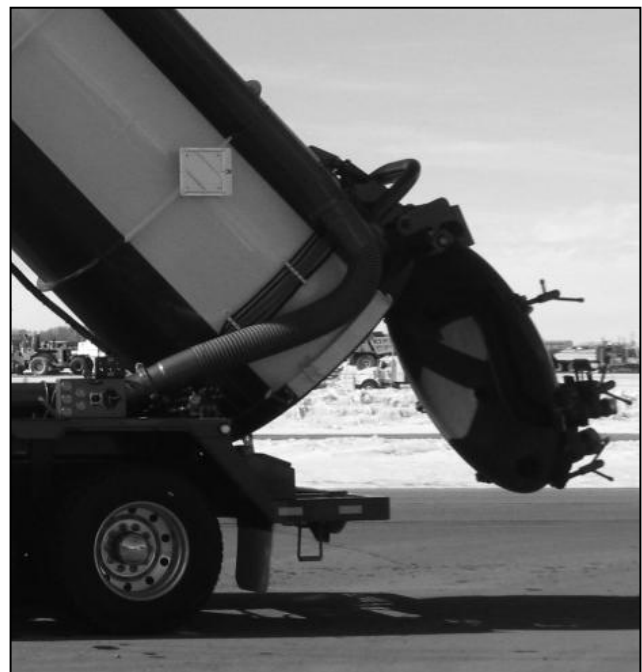
Photograph of the rear door configuration of a typical vacuum truck. Note crush point.
