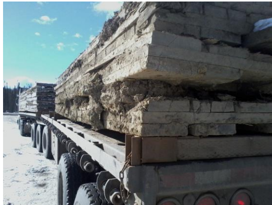
VIEW OF UNACCEPTABLE LOAD WITH MUD AND ROCKS ATTACHED TO MATTING
