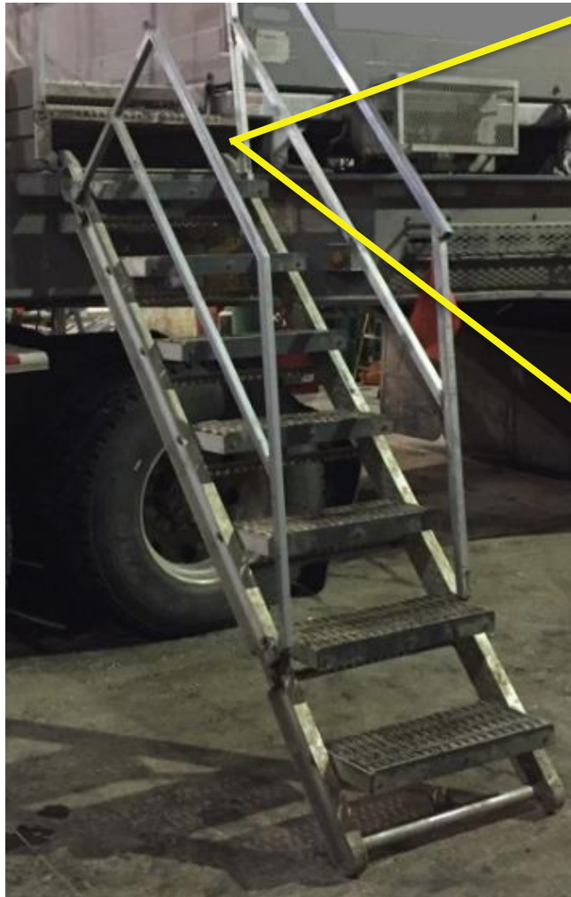
The stair stops, or “ears”, on the stow box are expected to hold the roller in place while in use. Note the roller is not secured behind the stair stops (red circle).
