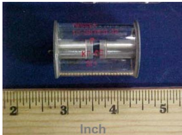
View of Spark Gap or "Electron Tube" Containing Radioactive Gas (Krypton-85) Photo provided courtesy of Unison Industries
