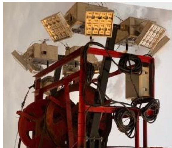
Figure E-12: Portable LED Lighting for Trucks, Work-over Rigs, Cranes, etc. (Photo courtesy of CLEANTEK Industries Inc.)
