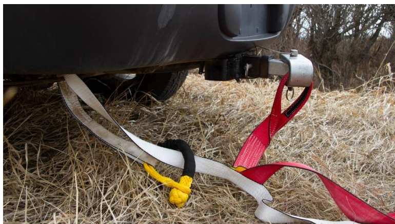
Figure 3.1: Attachment of a kinetic energy containment diffuser around frame with a soft shackle. Image courtesy of Cenovus.
