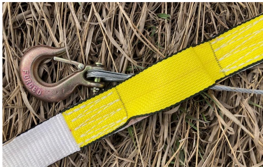
Figure 3.5: Kinetic energy containment diffuser used with winch lines. Image courtesy of Cenovus.
