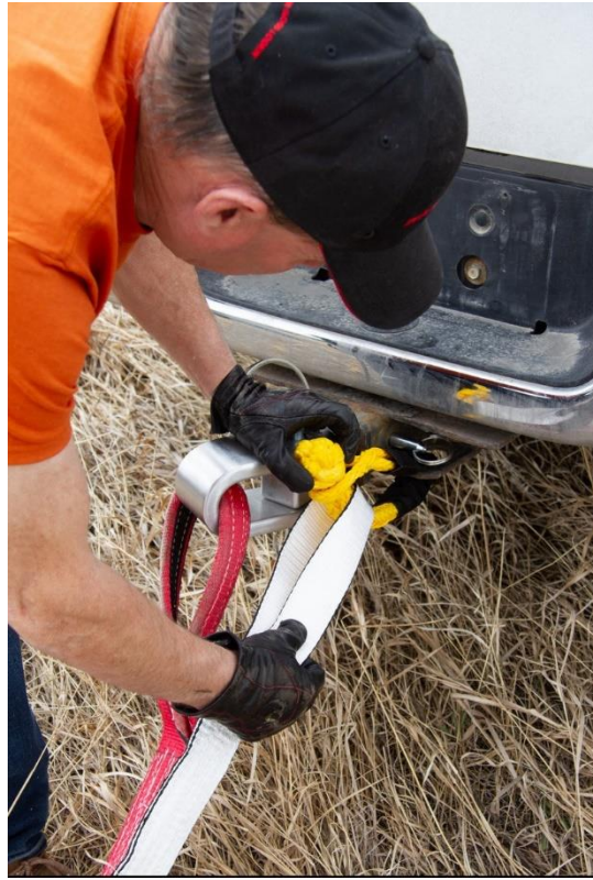
Figure 3.2: Attachment of a kinetic energy containment diffuser to hitch safety chain hole with a soft shackle. Image courtesy of Cenovus.
