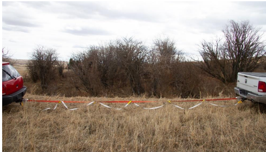
Figure 3.3: Kinetic energy containment diffuser using a tow strap. Image courtesy of Cenovus.
