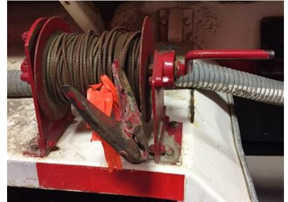
EXAMPLE OF A TRUCK BONDING CABLE REEL
