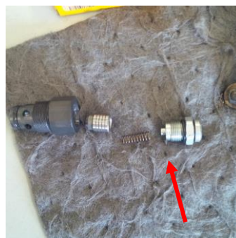
The proper order for the orifice to be assembled for use. Note location of the spring.
