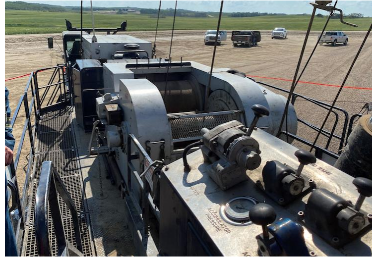
Typical rig hoisting equipment, draw works and drill line.
