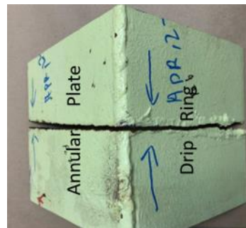
Failed annular bottom plate
