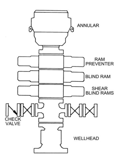
Figure 2. Elevated Sour Well Servicing BOP Stack with Shear Blind Ram
